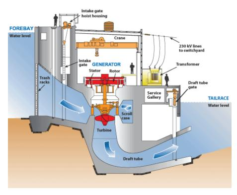
Water enters the station through the intake and enters into the scroll case. The **scroll case** is a spiral area surrounding the turbine. The movement of the water causes the turbine to spin.
